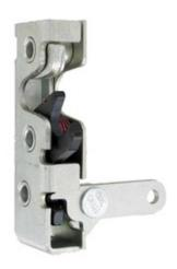
This compact single rotor latch is designed for light to medium applications for on or off-highway entrance doors, compartments and access panels. It features a variety of trip levers and mounting axles for ease of mounting and application and is FMVSS 206 compliant.
